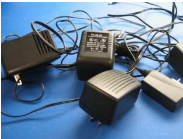
Figure 1. "Wall Warts" required for "Self-powered" PC peripherals
