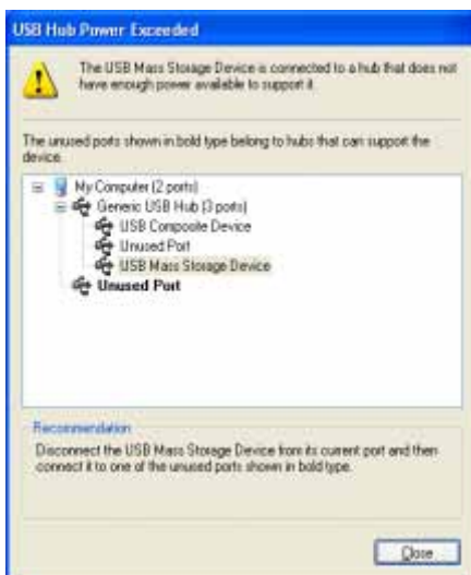
Figure 4. Port error by Windows XP when High Power port is unavailable
