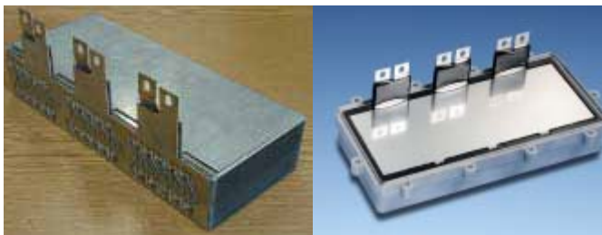
Figure 7: PCC, C_R=2mF , U_R=450VDC , L_xW_xH= 270x125x56mm^3 , water cooled, -40^\circ C up to +125^\circ C for the 1 st generation HEV converter.
