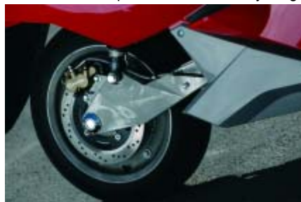
Figure 1. The electric motor is housed in this aluminium swingarm
