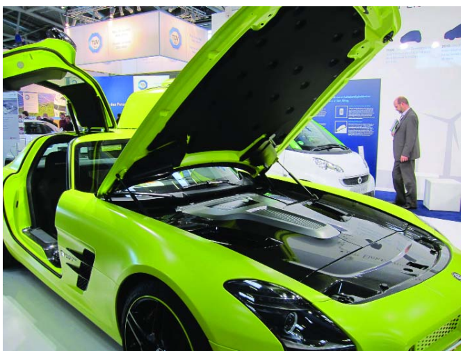
Figure 1: The Mercedes SLS AMG Coupé Electric Drive was one of the eye catcher of this year's eCarTec. The EV has four electrical motors and uses Li-Ion batteries. (Picture: Marisa Robles Consée)
