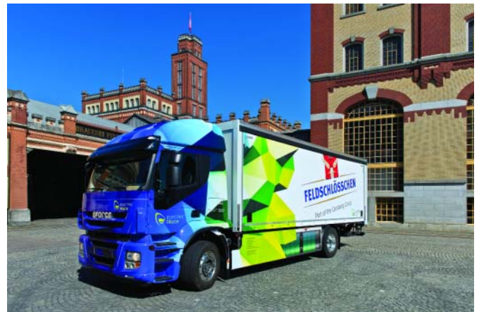
Figure 3: The electrical 18-tonne truck E-Force uses two Brusa electric motors, controllers and chargers as well as a DC converter. (Picture: Brusa)
