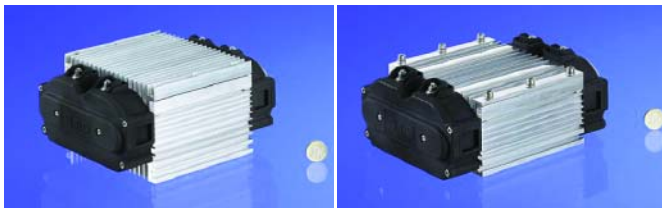
Figure 1: Power inductors optimized for 3m/s forced air cooling (a) and cold plate mounting (b)
