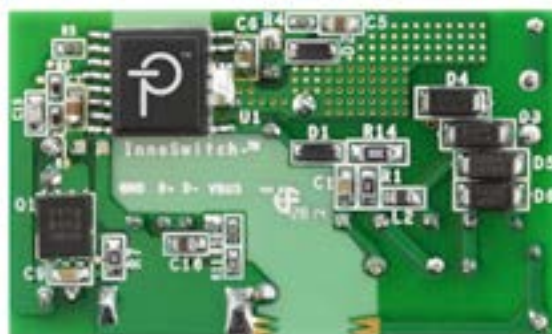
Figure 3: An InnoSwitch IC is placed across an isolation area
