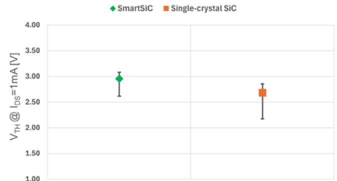
Figure 4: V_{th} comparison for a 13mOhm / 650V Gen2 SiC MOSFET manufactured in single-crystal SiC and SmartSiC™ substrates.
