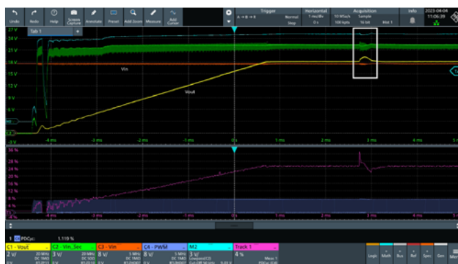
Figure 5: Startup of the converter and irregular control effects
