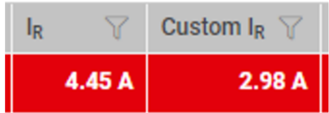
Figure 2: Datasheet Rated Current (left) and Custom Rated Current value (right) based upon dimension entered in the user interface.
