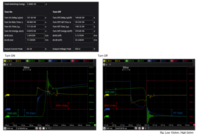
Figure 4: Test results (turn-on & turn-off) for a SiC MOSFET.
