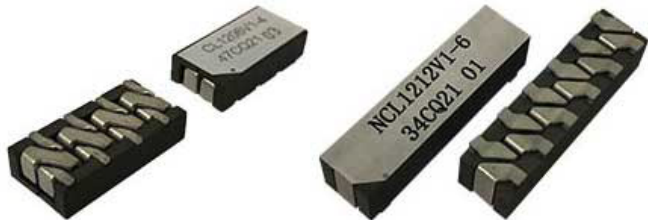
Figure 4: A series of coupled inductors commonly used with ADI's multiphase VR designs.
