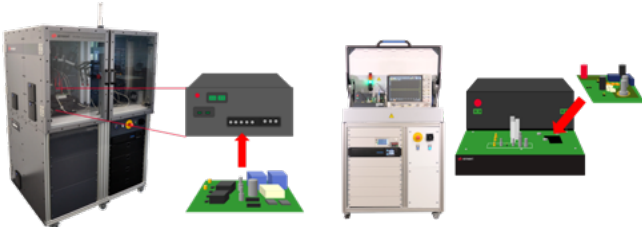
Figure 3: Tailored bare chip DUT fixture for PD1500A/PD1550A.
